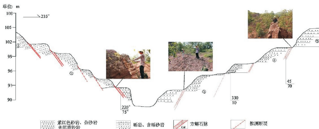
图8 十八罗汉山地形地质剖面图(1:500) Fig. 8 The geological profile of Luohanshan
