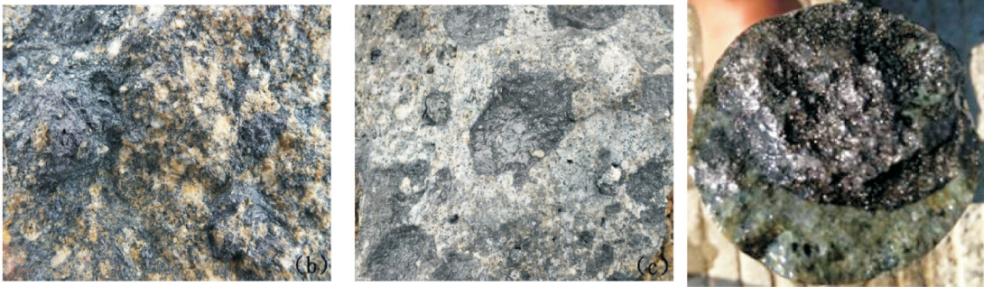
图9 ②号石墨矿体地表石墨构造形态特征(据野外照片) (资料来源于新疆奇台县黄羊山石墨矿调查评价项目, 2017年) a—石墨呈豆状、不规则细脉状、球状集合体;b—石墨呈球状、豆状及细鳞片浸染状;c—钻孔中的石墨呈球状、球斑状特征 Fig.9 Structural morphological characteristics of surface graphite of No. ②(after photos in the field) (Source of information: Research and evaluation project of Huangyangshan graphite ore deposit in Qitai County, Xinjiang, 2017) a- Lenticular, irregular and fine pulse, globular aggregate of graphite;b- Globular aggregate, lenticular and impregnation of fine scale graphite; c- Globular aggregate and ball-shaped graphite in drill hole
