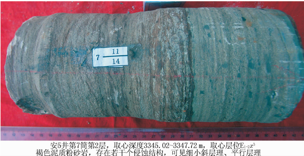
图 7 褐色泥质粉砂岩侵蚀结构 Fig.7 Brown argillaceous siltstone and erosion texture
