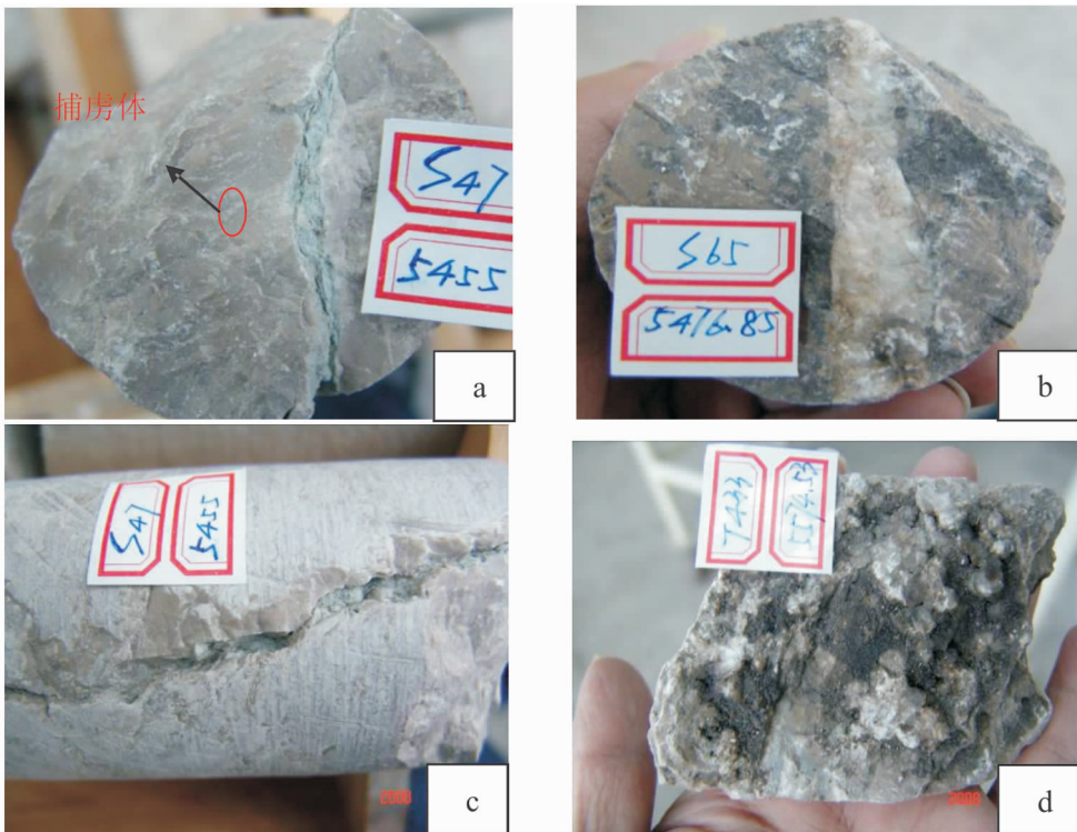
图 6 裂缝充填情况 Fig.6 Filling situation of the fissures
