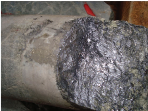
图 6 辉钼矿呈细脉状充填于变质岩裂隙中 Fig.6 Veinlet molybdenite filling fractures of metamorphite
