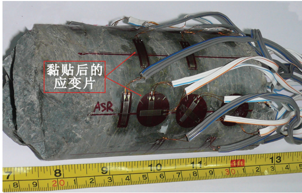
图2 粘贴应变片后的岩心 Fig.2 Rock core with strain gauges
