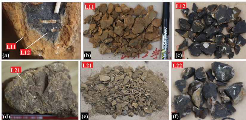
图7 烂泥沟滑坡的两组玄武岩样品 Fig.7 Two groups of basalt samples from Lannigou landslide
