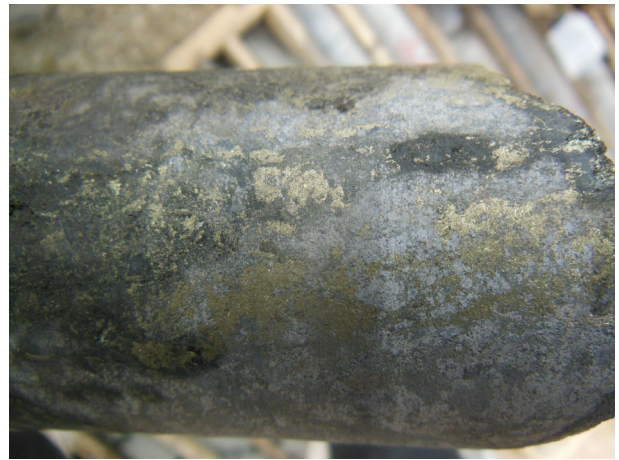
图7 ZK3中细脉浸染状黄铜矿 Fig.7 Veinlet disseminated chalcopyrite in ZK3
