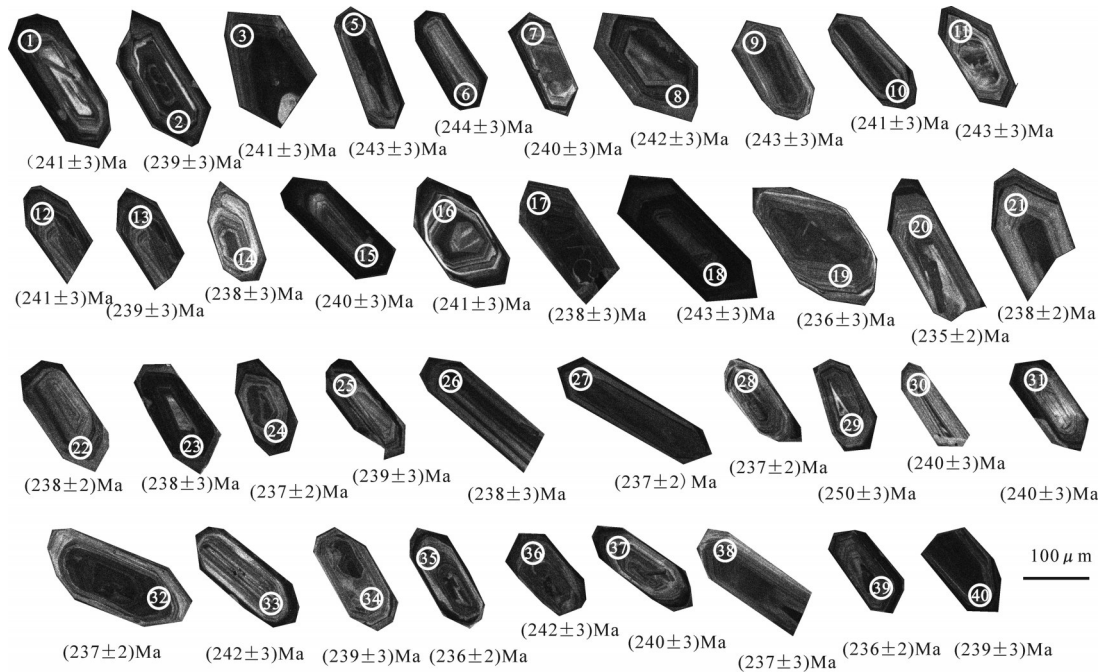
图4 大水沟英云闪长岩锆石阴极发光照片(圈内数字代表U-Pb分析点,其他数字代表 206 Pb/ 238 U表面年龄) Fig.4 CL images of zircons from Dashuigou tonalite (numbers in the circles represent analytical spots of U-Pb, and the values represent ages of 206 Pb/ 238 U)
