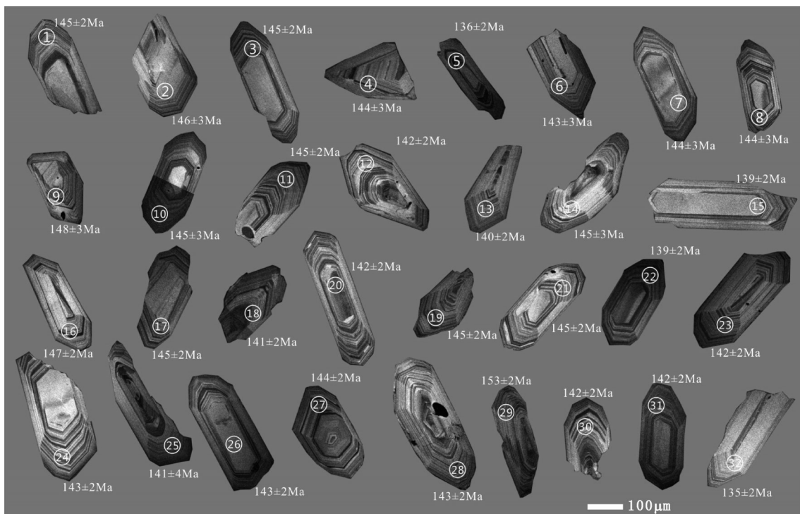
图10 虎山石英二长闪长岩(10CL523-3)锆石阴极发光图像 Fig. 10 Cathodoluminescence images of zircon of quartz monzodiorite (10CL523-3)
