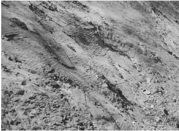
图5 滑床表部的反坡阶步现象 Fig.5 Antistep on surface of sliding bed
