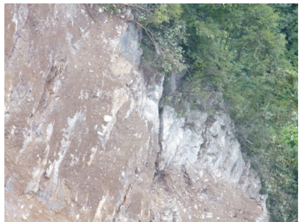
图8 剪出口左翼岩体张拉破坏特征显著 Fig.8 Outstanding tension deformation of rockmass on the left of rockslide outlet
