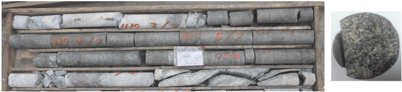
图9 魏墩验证钻孔岩心及铁闪锌矿矿体岩心断面图 Fig.9 Geological section of verification drill hole core and marmatite orebody
