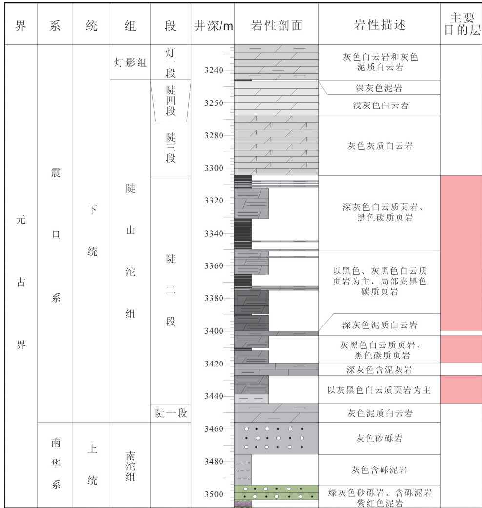
图2 鄂阳页1井震旦系陡山沱组地层柱状图 Fig.2 Stratigraphic column of the Sinian Doushantuo Formation, Eyangye1 Well
