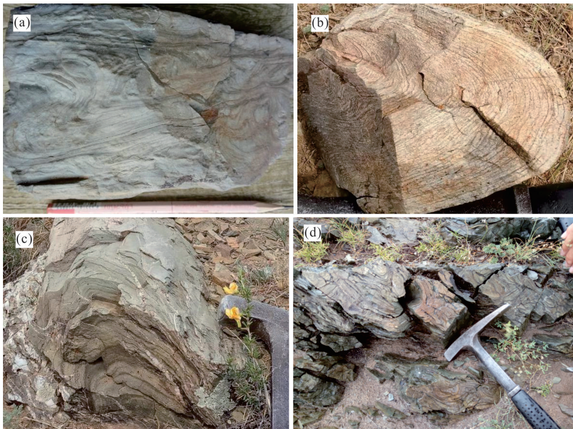
图6 乌兰敖包组变形褶皱构造 a—变质粉砂岩中滑动褶皱; b—变质细粒长石英砂岩中等厚褶皱; c—粉砂质板岩中的同斜倒转褶皱; d—韧性剪切带鞘褶皱 Fig. 6 Deformed fold structure of Wulanaobao Formation a – Strain-slip folding in the metamorphic siltstone; b – Isopach fold within the metamorphic quartz sandstone; c – Synclinal reverse fold in the slate; d – Sheath fold within the Ductile shear zone
