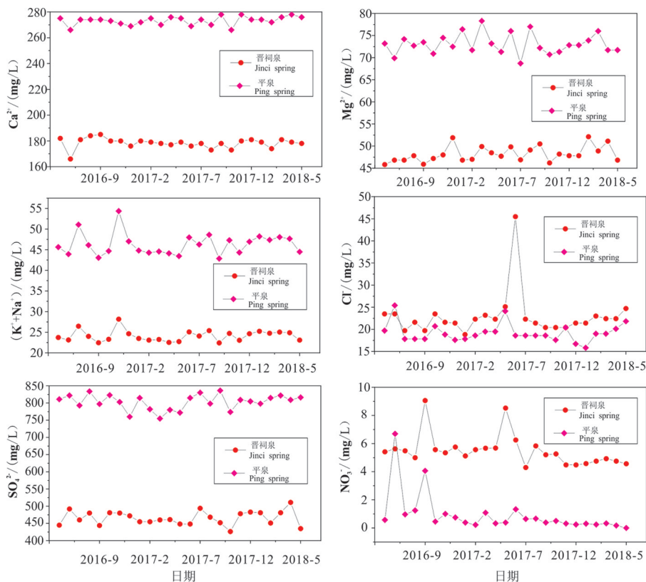
图6 晋祠泉及平泉水主要水化学组分含量月均动态 Fig.6 Monthly average dynamics of main hydrochemical components in Jinci Spring and Pingquan Spring
