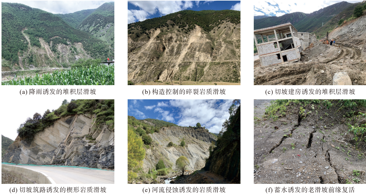
图 6 研究区典型滑坡类型 Fig.6 Representative types of landslides in the study area
