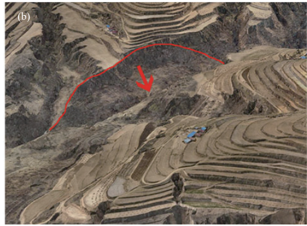
图 6 滑坡体色调特征(a—色调较浅, 镜头方向 22°; b—色调较深, 镜头方向 135°) Fig.6 Characteristics of landslide tone (a—Light tone, lens direction 22 °; b—Dark tone, lens direction 135 °)
