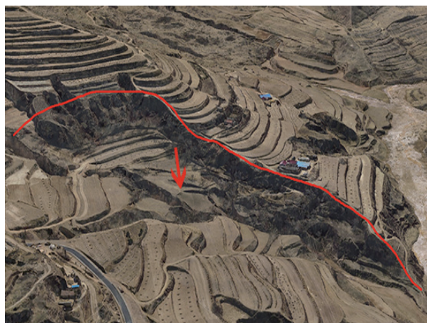
图 11 滑坡壁发育剥落和小规模坍塌(镜头方向 90°) Fig.11 Landslide wall development spalling and small-scale collapse (Lens direction 90°)
