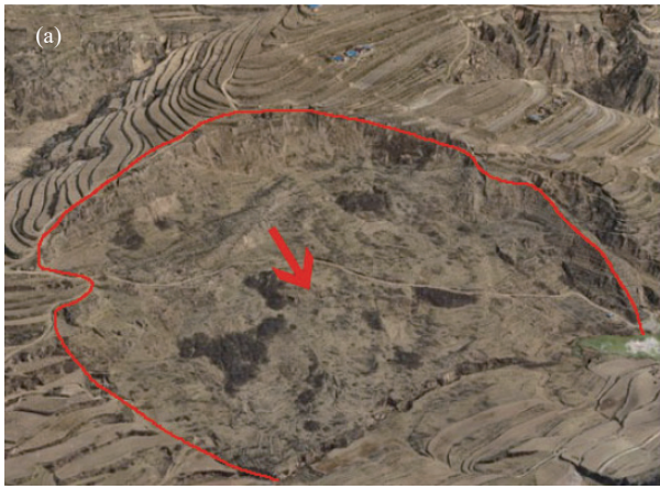
图 6 滑坡体色调特征(a—色调较浅, 镜头方向 22°; b—色调较深, 镜头方向 135°) Fig.6 Characteristics of landslide tone (a—Light tone, lens direction 22 °; b—Dark tone, lens direction 135 °)
